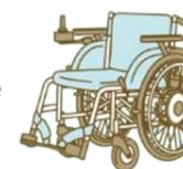
An electric wheelchair with a lightweight motor, etc. Operated by a joystick and can be switched between electric and manual operation
