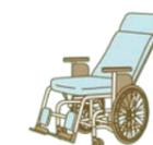
The angle of the seat and the back can be changed to resting and other positions. Some electric wheelchairs have a function to change sitting positions.
